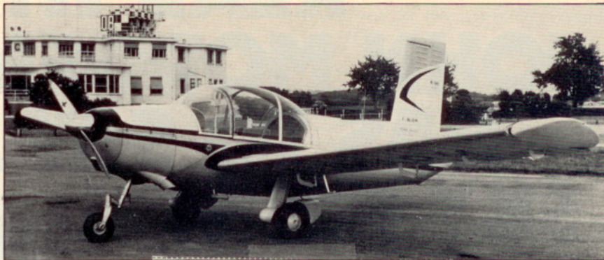
The Rallye taildragger has come a long way from its first-born cousin (above), a three-seat, tricycle gear aircraft powered by a 90-hp Continental engine.
