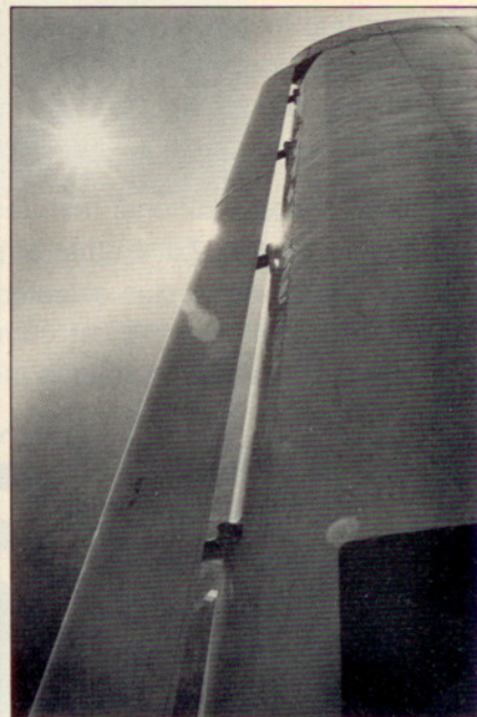
The slats remain flush against the wing in normal flight, but extend down and out at high angles of attack and enhance the airplane's low speed handling.
